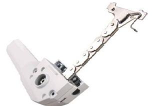
This inconspicuous Teleflex-clearline opener features a fully retracting stainless steel chain with quick release window attachments to facilitate window cleaning. With an internal projection of 64mm the enclosed chain case permits ease of operation whilst allowing close fitting of curtains or blinds.
